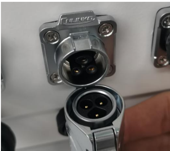
Step5: This is the socket for the RES handle, align the inserts and push it in.
