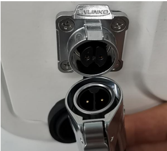
Step3: The first is two RES eye handles, the same plug-in, align the socket on the back of the machine, and push it in.
