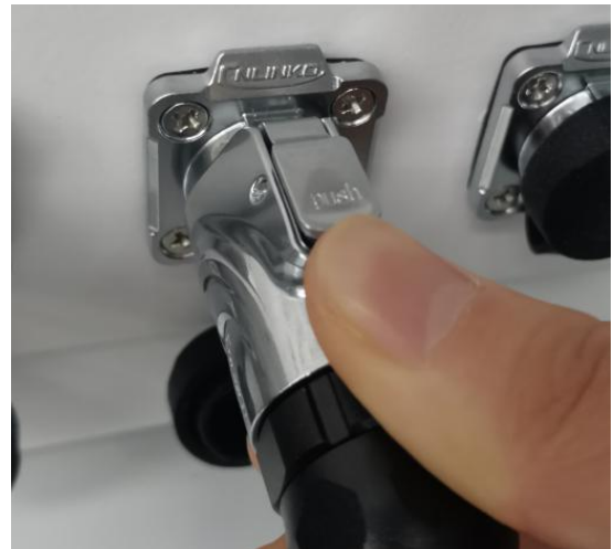
Step5: This is the socket for the RES handle, align the inserts and push it in.
