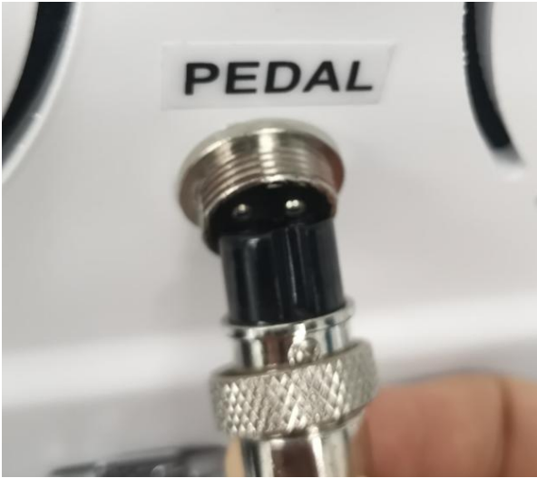
Step1: Insert the footrest into the socket.
