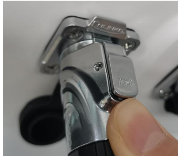
Step3: The first is two RES eye handles, the same plug-in, align the socket on the back of the machine, and push it in.
